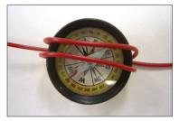
If you don't have an ammeter, simply wrap the wire around a compass, and watch the needle deflect as you pass the magnet in and out of the coils, as shown in the image at left.
